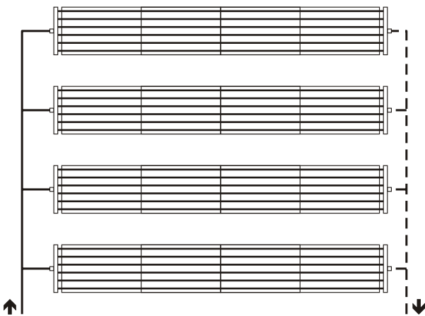
Fig.19 ECOPAN radiant panels in parallel with opposite connections
